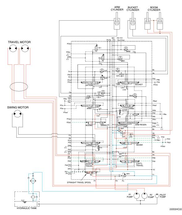
When the boom and travel functions are operated, simultaneously the boom spools and travel spools in the main control valve are moved to the functional position by the pilot oil pressure from the remote control valve and the straight travel spool is pushed to the right by the oil pressure from pilot pump.
